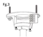
Place fan into hanger bracket and align Ball Joint Slot with hanger bracket as illustrated.(See Fg.3)
