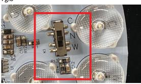
Choose colour temperature by flicking the switch in the LED (See Fg.10)
