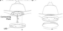
**To install:** Remove the screw from the connecting plate. Plug the wire into the light kit mounting hole. Align the thread with connecting plate before tighten the screw.
