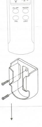
Installation of Transmitter Wall Mount Holder with two screws.
