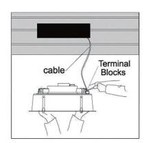
Cut around the attached hole-cutting template and use this template to mark the hole outline on the ceiling.
