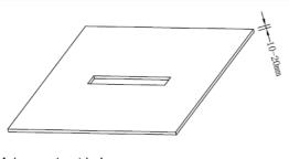
1, Make a cut out hole, The thickness of mounting plate 10 to 20 mm.
