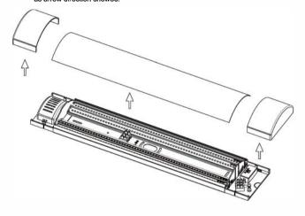
Step 3: The 2nd method of Installation: Wire the AC cable into the terminal block through the cable entry hole at the base housing or end cap. Mount the fitting onto flat service with wall plugs and screws.
