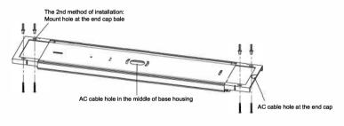
Step 5: Assemble LED diffuser back to base housing.
