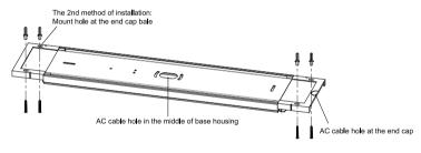
Step 5: Assemble LED diffuser back to base housing. Setting the desired color temperature on the switch.
