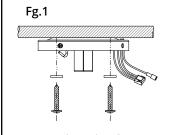
Secure the ceiling fan mounting plate to the ceiling using screws and washers provided. Ensure screws are tightened on the mounting plate.
