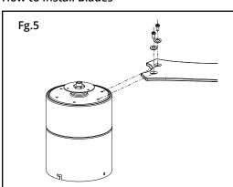
Attach the blade to the top of the motor. Tighten and secure blade with screws and washers provided. Repeat this procedure until all blades are installed.
