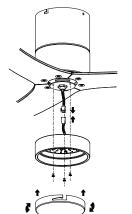
Connect the 2-pin connectors from motor housing with the light kit plate.
