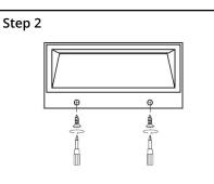
Unscrew and remove the mounting bracket.
