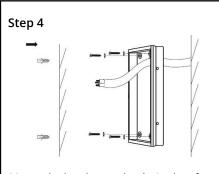
Mount the bracket on the desired surface using the four screws supplied.
