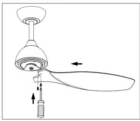
Install the blades to the bottom of the motor. Tighten and secure blade with screw and washer provided. Repeat this procedure until all blades are installed.
