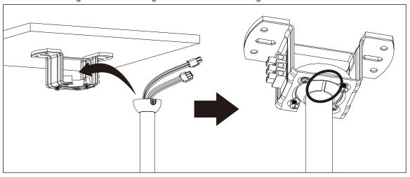
Place the receiver into the bracket and connect between power and motor as illustrated.
