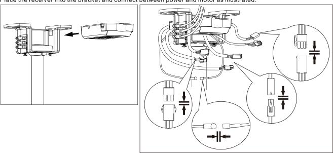
Wire up the receiver with quick connectors and insert into the mounting bracket. Please make sure the antenna wire has been safely folded inside the canopy cover before final assembly (DO NOT cut the antenna wire)
