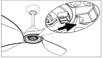
Connect LED with power by the quick connectors.
