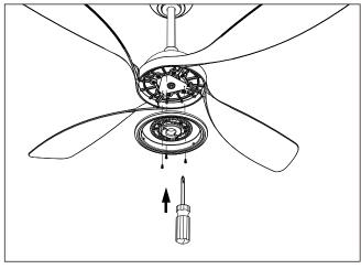
Install the LED light plate onto the steel bracket as illustrated with the 3 supplied screws.
