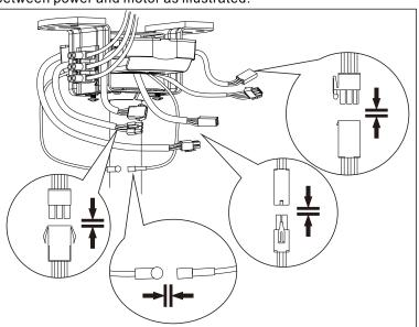
Wire up the receiver with quick connectors and insert into the mounting bracket. Please make sure the antenna wire has been safely folded inside the canopy cover before final assembly (DO NOT cut the antenna wire)
