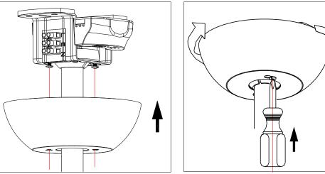
Carefully put the screw cap on using the piece of magnetic supplied.
