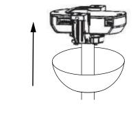
Slide the canopy upward onto the mounting bracket and rotate it counter-clockwise to lock it in place. Verify that both mounting bracket tabs are fully engaged within the canopy slots. The canopy should have an approximate 3mm gap from the ceiling.
