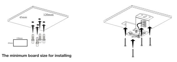
Align the bracket and screw the hanger bracket to the ceiling tightly.
