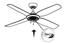
Plug the plug from light kit into the plug from the fan.
