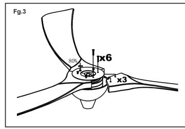
Install the blades and blade fixing metal plate to the motor with screws provided, first tightening the screws by 80%, Repeat this procedure until all the blades are installed, and then tighten the screws fully.
