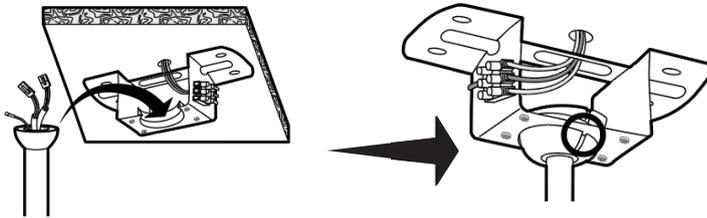
Place fan into hanger bracket and align ball joint slot with hanger bracket as illustrated.
