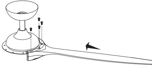
NB: Ensure the blades do not get damaged or bent during the installation process while the fan is on the ground. This will affect the performance and balance of the fan and this is NOT covered under warranty.
