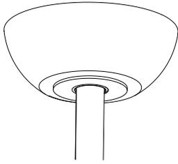
After wiring is completed, attach the canopy to the hanger bracket by pushing upwards and twisting anti-clockwise. Tighten screws and ensure canopy is not touching the ball joint.
