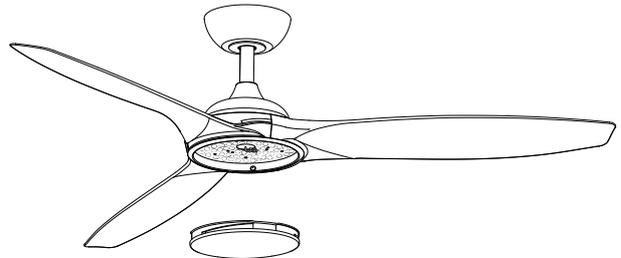
Align the convex point on the light plate with the gap on the LED mounting plate and press down firmly.
