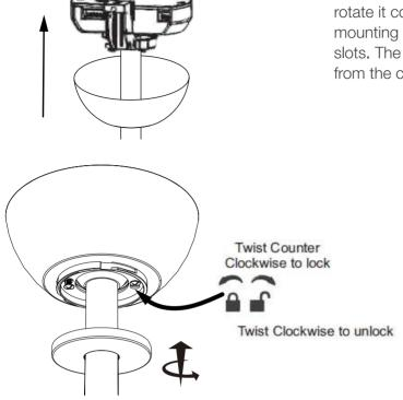
Slide the canopy upward onto the mounting bracket and rotate it counter-clockwise to lock it in place. Verify that both mounting bracket tabs are fully engaged within the canopy slots. The canopy should have an approximate 3mm gap from the ceiling.
