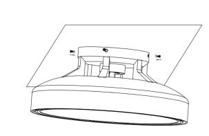
4. Put the lamp on the mounting plate, align it with the hole and fix it with screws.
