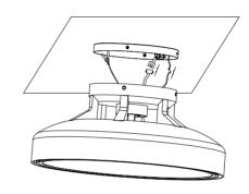
3. Hang the wire rope on the hook of the mounting plate of the lamp, and plug the power cable terminal into the pair, and then plug the ground terminal into the pair.
