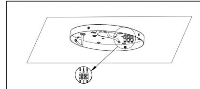
2. Connect the wires to the terminal block, as shown in the Figure.
