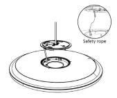
Step 3. Hang the safety rope then connect the power cord.
