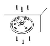
Step 2. Fix the hanging plate to the ceiling
