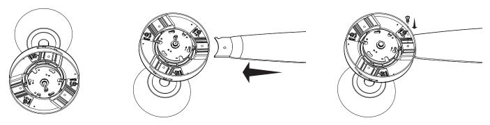
**WARNING**: This Fan has click in blades, it is essential that the installing <u>electrician has applied an appropriate</u> <u>amount of force to ensure the blades are clicked in securely before engaging the screw and before turning the fan on.</u> This is to ensure the blade is secured, and in the case of a defective spring latch. Martec will not be responsible for any consequential damage because of this.
