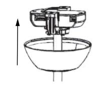
Slide the canopy upward onto the mounting bracket and rotate it counter-clockwise to lock it in place. Verify that both mounting bracket tabs are fully engaged within the canopy slots. The canopy should have an approximate 3mm gap from the ceiling.
