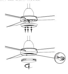
Align the convex point on the light plate with the gap on the LED mounting plate and press down firmly.
