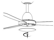
Twist to install the bottom plate
