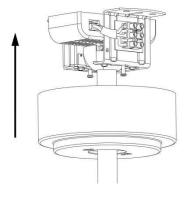
Slide the canopy upward onto the mounting bracket and rotate it counter-clockwise to lock it in place. Verify that both mounting bracket tabs are fully engaged within the canopy slots. The canopy should have an approximate 3mm gap from the ceiling.
